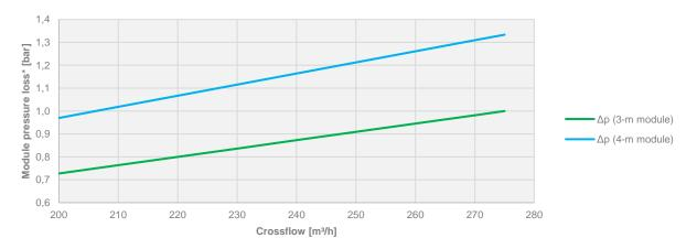
\* The module pressure loss value include the pressure loss of the corresponding U-bend. The data is representative for water or similar viscosity liquids.
